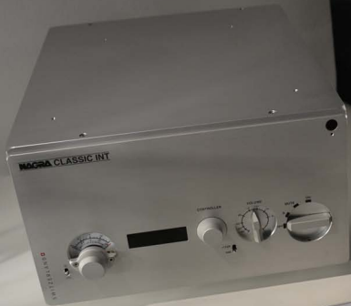
NAGRA Nagra CLASSIC INT Stereo integrated amplifier 2x 100 W rms into 8 Ohms
